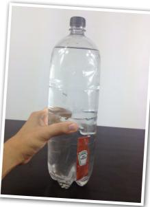
When you squeeze the bottle this increases the pressure! This squashes that little pocket of air inside the sachet making it more dense so it starts to sink. When you let go of the bottle, the air inside the sachet spreads back out and the sachet gets bigger (making it less dense) and so your submarine rises back up to the surface!
