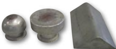
In testing, the hemispherical and flat anvils are the two most crucial
